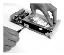
7. Pressing down the hard drive and tighten all 4 screws to secure the hard drive to the Base Plate.
